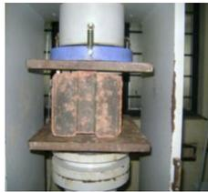
**Fig.2.** Test set-up for compression test
